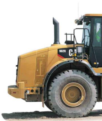
FIGURE 1. THE WHEEL LOADER ENGINE COMPARTMENT WITH CONE AND CYLINDRICAL EXHAUST STACK
