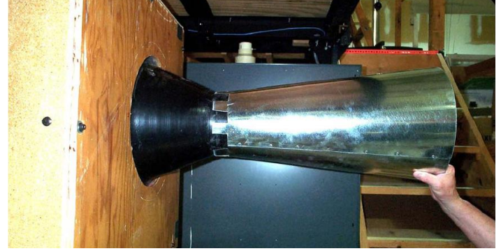
FIGURE 9. ELEVATION VIEW WITH DIFFUSER CONE ATTACHED TO CAT CONE
