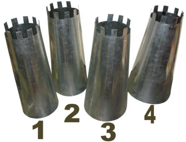
FIGURE 6. PHOTOGRAPH OF THE FOUR DIFFUSERS USED IN THIS STUDY
