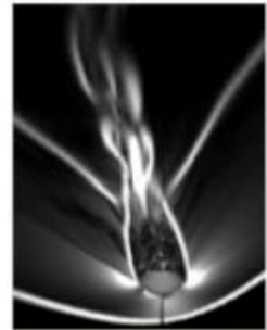
Fig. 1 Dynamic instability Analysis of the Hayabusa capsule
